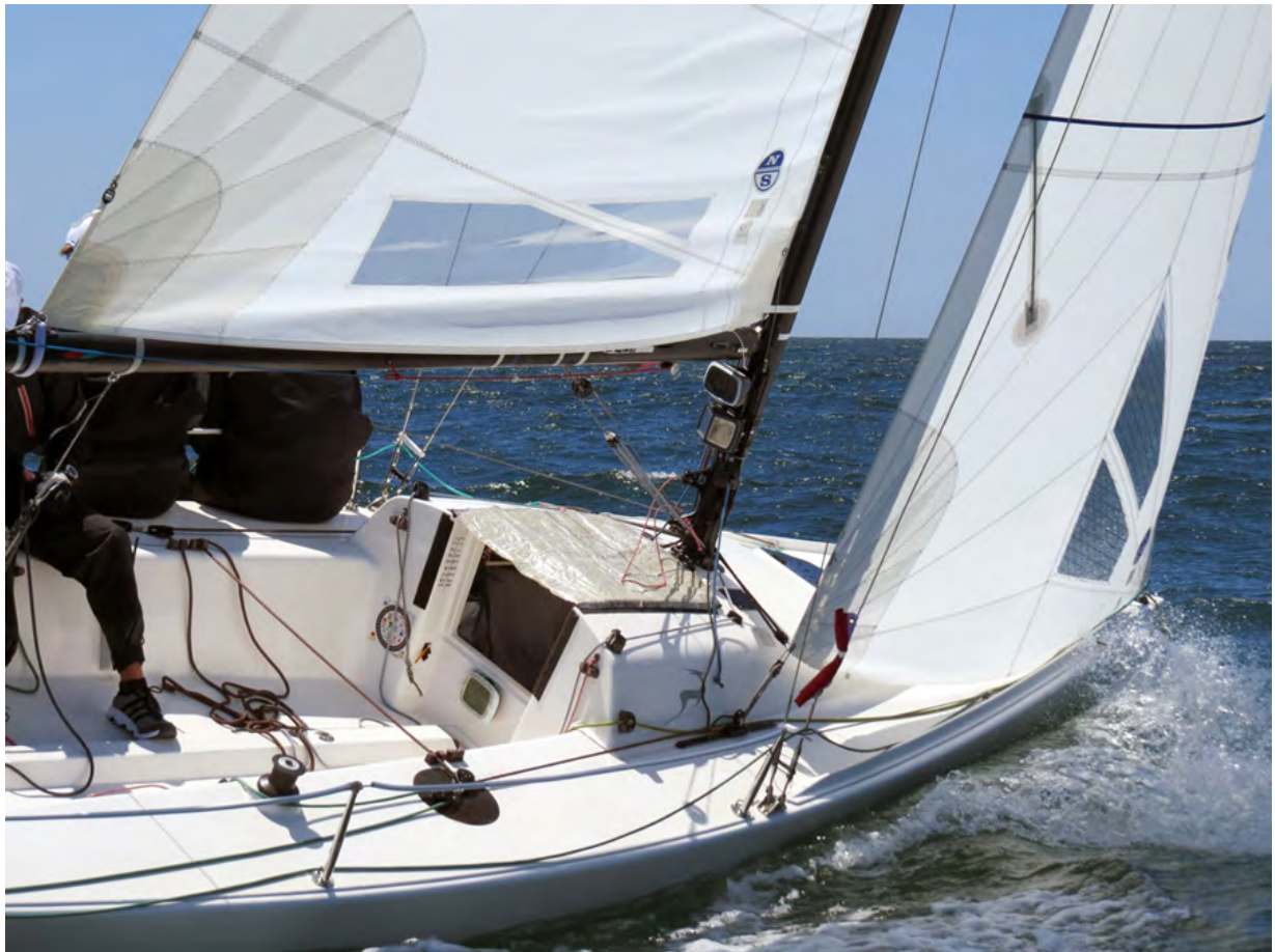
Teams often trim the jibsheet to windward, using cam cleats mounted on each side of the cockpit.
