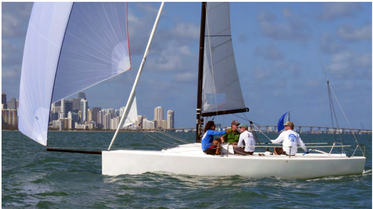
In light air downwind, the crew is far forward—helm against winch, two against the bulkhead, and one ahead of the shrouds but not in front of mast (per class rules).
