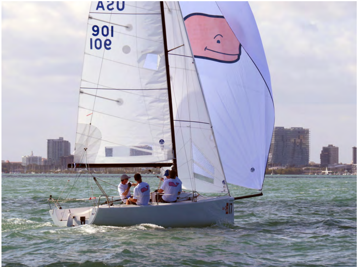
After the set, the jib is being furled. This boat is sailing low, in displacement mode.
