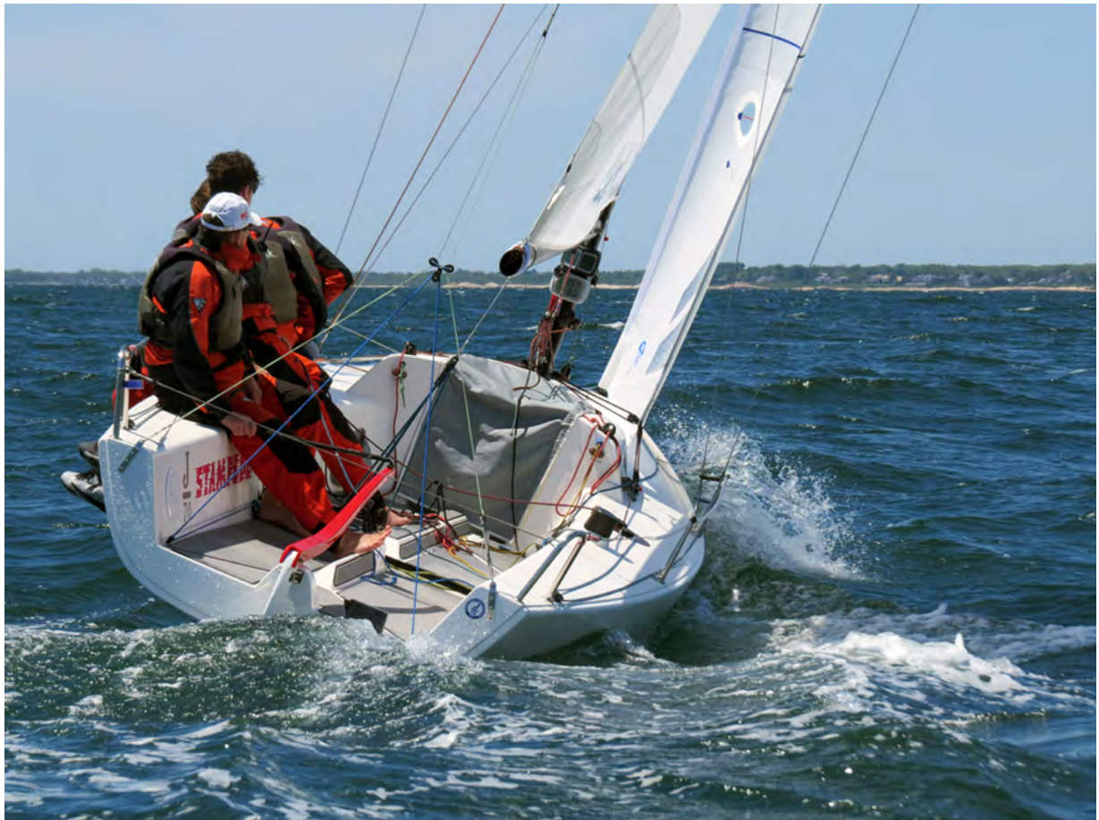
Upwind trim typically includes tightening the in hauler (windward sheet), which moves the jib lead to windward and reduces sheeting angle. If it gets too choppy, ease the sheet and move the jib lead forward.
